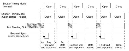
Figure 34. LightField Clean Until Trigger (CUT) Timing Diagram
